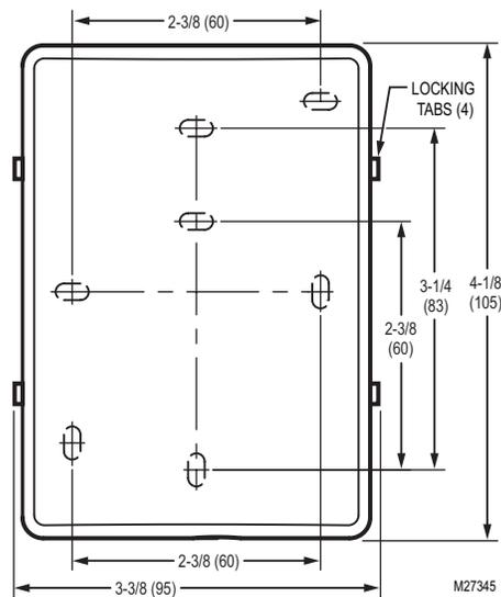
Fig. 2. Subbase mounting holes and locking tabs.
