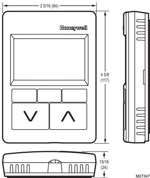
Fig. 4. LCD Wall Module dimensions in inches (mm).
