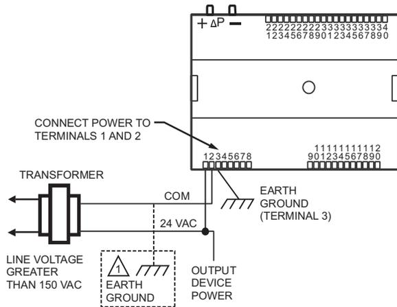
**⚠ IF THE CONTROLLER IS USED IN UL 1995 EQUIPMENT AND THE PRIMARY POWER IS MORE THAN 150 VOLTS, GROUND 24 VAC COM SIDE OF TRANSFORMER SECONDARY.**
