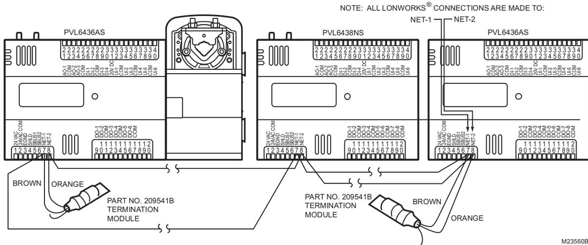
Fig. 14. Termination modules (LoNWORKS® daisy chain connections).
