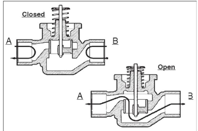
Fig. 2 - Fluid flow of 3-way valves
