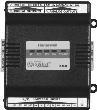
The on-board I/O can be used to monitor pulse contacts from power/demand meters, analog sensors, or transducers, as well as to control energy-consuming devices such as fans, lights or pumps with digital relay outputs. Also included are 4 analog outputs to proportionally control dampers, valves and other devices.
